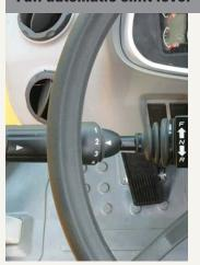
A single lever on the left side of the steering column gives the operator fast, easy control of speed and direction. Push the lever forward to go forward, pull it back for reverse. Travelling is automatically changed from 1st stage to given stage according to travel speed and tractive effort. The operator can select two kinds of automatic modes (1st ↔ 4th, 2nd ↔ 4th).
